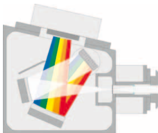
Optical design of the CAS 140CT based on an optimized crossed Czerny-Turner spectrograph
