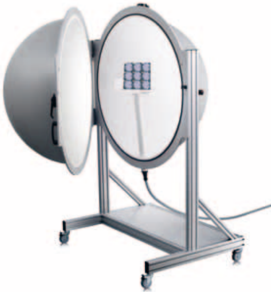
The ISP 1000 integrating sphere with 1 m diameter
